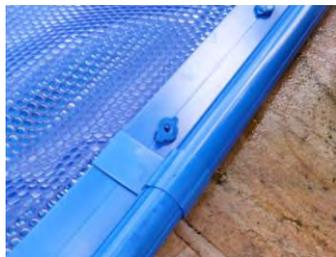
7. Take the 2-pronged part of the SmartClic and press it firmly through the pre-drilled holes and into the cover.
