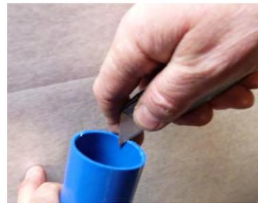
3. Then, using a sharp knife put a small mitre on the internal diameter of the tube. This will make it easier to push the sections together.
