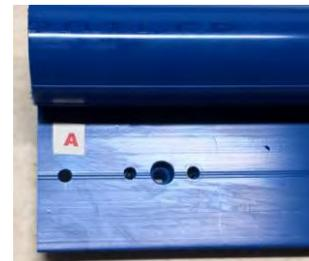
9. For high ambient and pool temperatures, the air in the flotation tube may expand and partially push the sections apart. To resolve this, labels A and B highlight pre-drilled holes. Push sections together again and using a 6mm drill bit, drill through from underneath the AquaSpoiler and come out of the top. Connect both sections using nuts, bolts and nut covers supplied.
