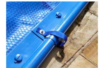
10. Attach the strap to the middle of the centre section and clip on the tow rope. The tow rope can be unattached and safely stored away when the pool is in use
